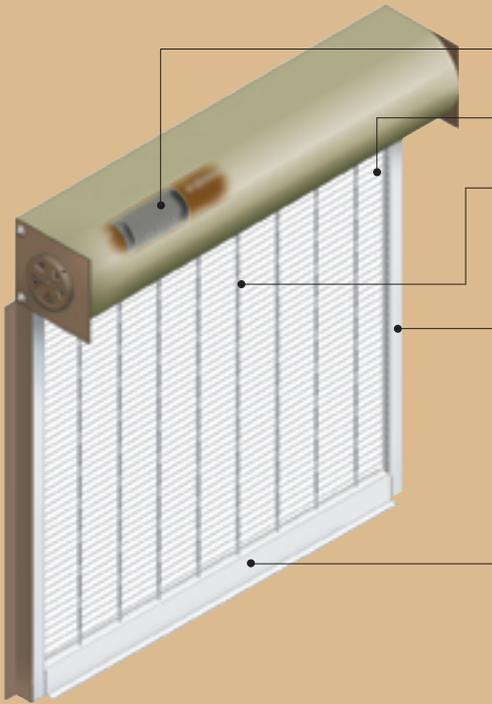
Oil Tempered Torsion Springs Designed for 50,000 Life Cycles
