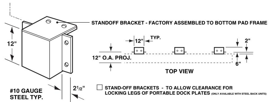
STAND-OFF BRACKETS - TO ALLOW CLEARANCE FOR LOCKING LEGS OF PORTABLE DOCK PLATES (ONLY AVAILABLE WITH STEEL BACK UNITS)
